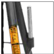
PIN IS FASTENED TO BODY BY A TETHER
